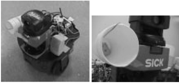
Figure 5. Left: A fully equipped Pioneer robot. Right: Close-up of the sensors. The microphone is glued to the bottom of two Styrofoam cups to add directionality.
