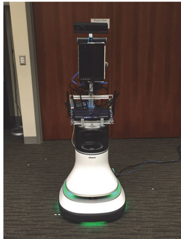
Figure 1: iRobot Ava Mobile Robot Platform with custom mobile remote presence interface and Microsoft Kinect sensor.
