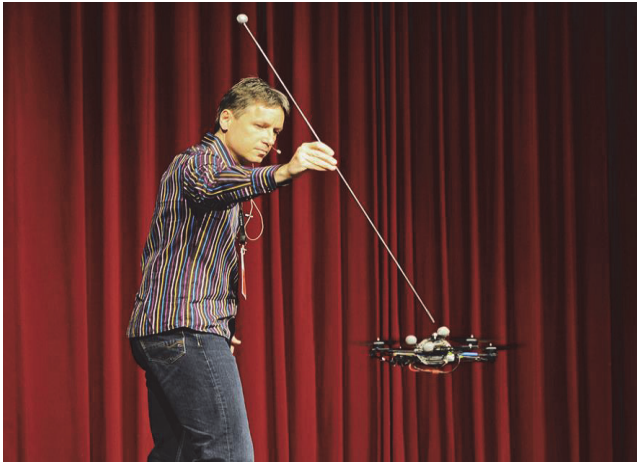
Figure 9: Demonstration of a flying inverted pendulum.
