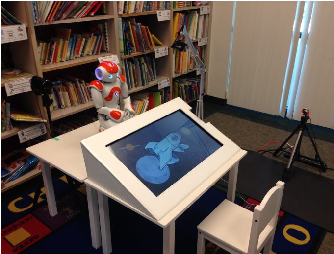
Fig. 2: The SAR system setup in preschool classroom. The system consists of a Aldebaran NAO robot and a touch-enabled tablet. All system content is openly available for research purposes; see Appendix.
