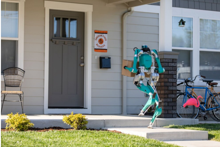
Figure 4.2: The Digit-1 robot developed by Agility Robotics for last mile delivery (Source: Agility Robotics)
