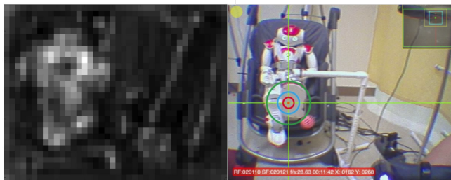
Fig. 2. Left: The surprise values of each 16x16 patch of pixels. Lighter pixels indicate higher surprise values. Right: Study environment from the infant's point of view with overlaid target to show infant gaze location during a robot kicking behavior. The circles indicate 2, 4, and 8 degrees from the estimated gaze location.
