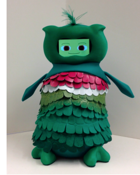
Fig. 1. SAR system used as the robot tutor: a SPRITE with the Kiwi skin.
