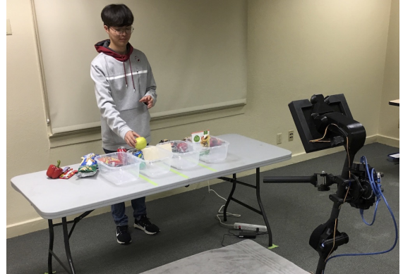
Fig. 1. Example interaction task in which a robot operator can use deictic gesturing for more efficient communication between their telepresence robot proxy (bottom right) and a teammate co-located with the robot (top left).
