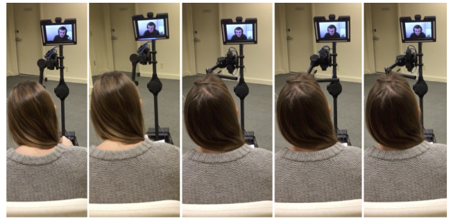
Fig. 4. Left: Basic robot mode. Second from Left: LED light mode; the activated blue LED lights pictured at the bottom of the robot’s screen moved around the screen in a standing pattern. Remaining Panels: Three frames from the arm motion mode; the robot’s arm moved in a similar way to a human performing beat gestures.
