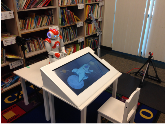
Fig. 1: The SAR system setup in preschool classroom with the Aldebaran NAO robot, a Lenovo IdeaCentre Horizon 27" touch tablet, a high-definition camera, and two webcams for multimodal data collection
