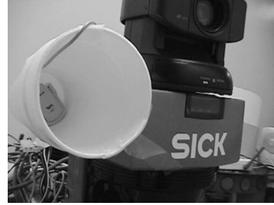
Figure 2: A close-up of the sensors. The microphone is glued to the bottom of two Styrofoam cups.
