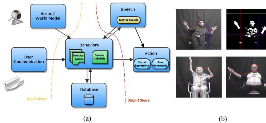
Fig. 2 (a) System architecture. (b) Visual user arm pose recognition algorithm output [24].
