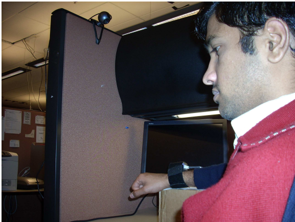
Fig. 3. A participant performing the WMFT assessment. The participant is being monitored by an overhead camera and an IMU on the wrist.
