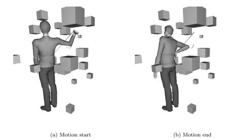
Fig. 1. Start and end of a motion generated by a linear hand trajectory with least-squares inverse kinematics. Paths to be taken by the hand and elbow are drawn.
