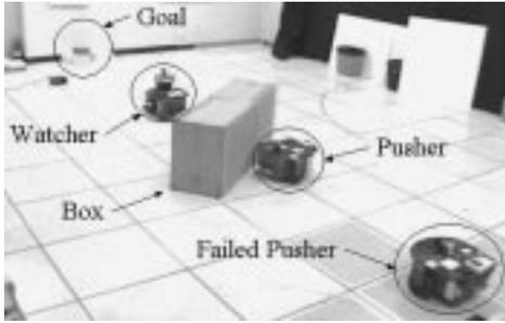
Figure 3: *Fault-tolerance in action: after we induced a single robot failure, the remaining robot is left to push on its own. (Image 2 of 3 taken from an experimental trial; see Figures 1 & 4.)*
