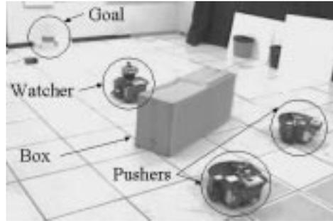
Figure 1: *Our experimental box-pushing setup. The task is for the pushers to move the box to the goal with the help of the watcher. (Image 1 of 3 taken from an experimental trial; see Figures 3 & 4.)*
