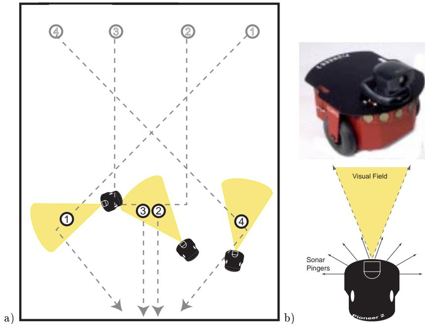
**Fig. 2.** a) *Experimental Environment*: The 18 by 22 foot corral. Robots are shown with observation ranges; fields of view extend further in a similar cone. Targets are numbered circles. Light grey targets and dashed lines indicate initial positions and paths of targets. b) *Robotic Testbed*: Three Pioneer 2DX robots.
