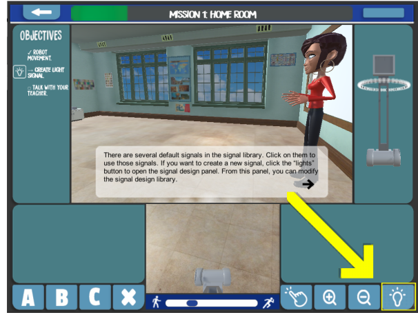
Fig. 3. The interface and robot are modeled after the Suitable Beam+. The interface has the same layout and camera views as the Beam+, but contains additional options for game play and the robot contains extra lights for signaling.
