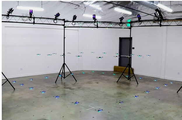
Fig. 5. Forty-nine Crazyflies flying in a 4-layer rotating pyramid formation. The bottom layer is 3 \text{ m} \times 3 \text{ m} with 0.5 m spacing between vehicles.
