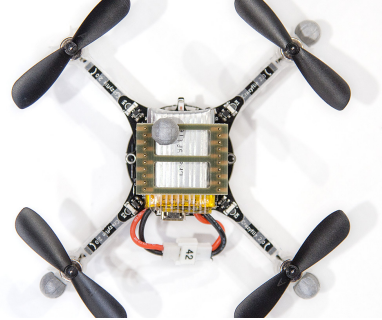
Fig. 1. The Crazyflie 2.0 miniature quadcopter with four motion-capture markers, LED expansion board (not visible), and battery.
