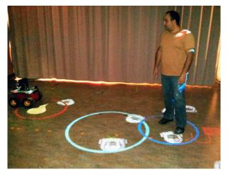
Figure 2. A person and a Pioneer 2AT collaborating on the herding task. The light bulb, pen, and lock are used to play the game. Circles are drawn around the robot and the person (red and blue, respectively).
