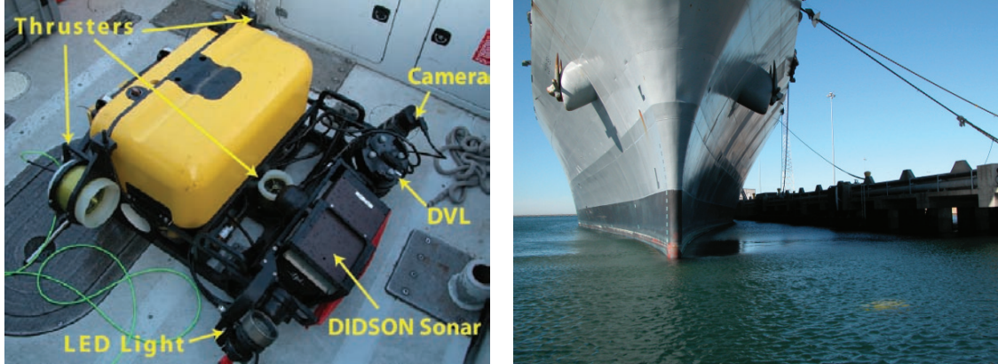
Fig. 2. Components of the Bluefin MIT-HAUV (left) and example deployment for inspection (right). The vehicle utilizes a DIDSON sonar to gather range scans of the ship hull. Localization is provided using a Doppler Velocity Log (DVL) assisted by an IMU. The thrusters provide fully actuated navigation and station-keeping capabilities.
