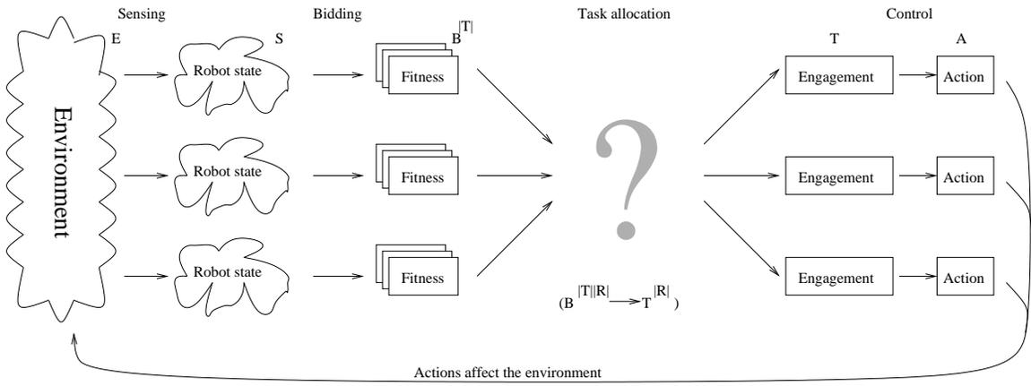
Figure 1: Reducing dimensionality of multi-robot coordination.
