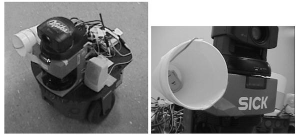
Figure 5: Left: A fully equipped Pioneer robot. Right: Close-up of the sensors. The microphone is glued to the bottom of two Styrofoam cups.
