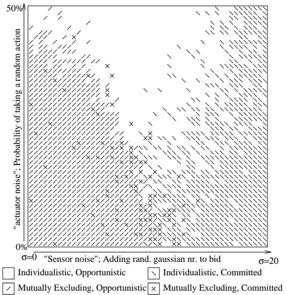
Figure 8: A cut through the parameter space of the grid world multi-robot emergency handling task. The graph shows the best performing strategy for each of  $50 \times 50$  settings, obtained by varying “sensor noise” and “actuator noise” parameters.
