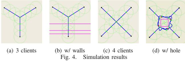
Figure 4(a) shows the result for three clients. Notice how the mother ships converge on the centroid of the triangle, and the robots are deployed at regular intervals along the medians, as expected. Figure 4(b) shows the output when the configuration is the same as figure 4(a) but with the addition of a wall. Since a wall attenuates radio signals, robots are deployed more frequently on the segment crossing the wall.
