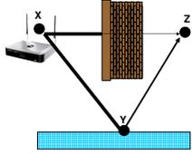
Fig. 2. Triangle inequality does not hold for path loss
