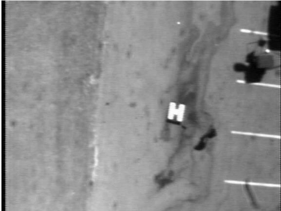
Fig. 3. An typical image obtained from the downward pointing camera on the helicopter during one of the trials. The landing target is the H shape.
