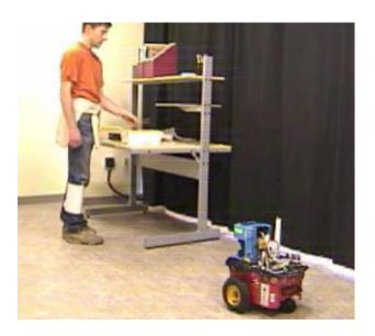
Figure 3: The experimental setup. The shown participant is performing task 1 (pencils) with the robot at a social distance. The laser fiducial is visible on the participant's leg. The motion sensor is mounted on the participant's left upper arm, and thus is not visible in this image.
