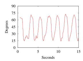
Figure 2: Example data from a motion sensor attached to a person's upper arm. As the person moves his arm up and down, the sensor reports the arm's angle in real-time.
