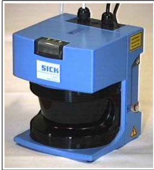
Figure 5.2. The laser range finder SICK LMS200
