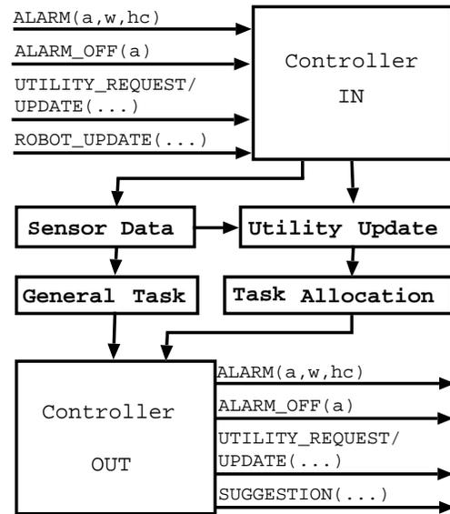
Fig. 2. Generalized Node Architecture.
