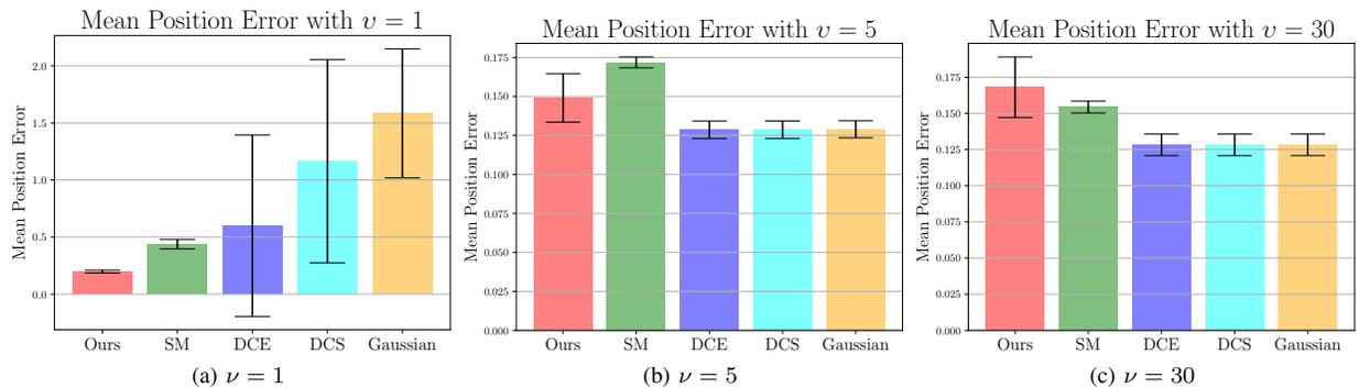
Fig. 1: Figure showing the results for the t-Student range sensor noise. Here we use  $\nu = 1$ ,  $\nu = 5$ ,  $\nu = 30$
