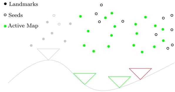
Fig. 3: The extraction of the *active map*. For the current frame (red triangle), we find the keyframes that have overlap with it (green triangles). Then the landmarks that are visible in these keyframes are extracted as the active map (green solid dots). Keyframes that have no overlap (gray triangles) and seeds (circles) are not considered in the active map.
