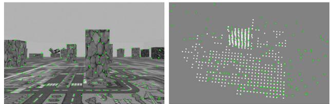
Fig. 4: An example of the *active map* and *dense map*. The left one is the image from the camera, where the solid green dots are *landmarks* and the circles are *seeds*. The right one shows the corresponding active map (green) and the dense map (white).
