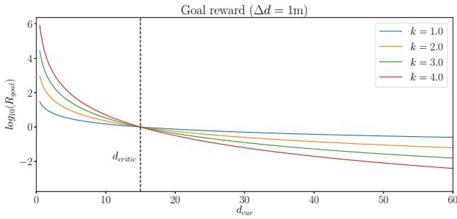
Fig. 8: Goal reward function when  $d_{\text{critic}} = 15\text{m}$ ,  $\Delta d = 1\text{m}$ . For the same  $\Delta d$ , the goal reward is higher when the quadrotor is close to the goal. When the distance to goal is smaller than  $d_{\text{critic}}$ , the goal reward increases more rapidly.
