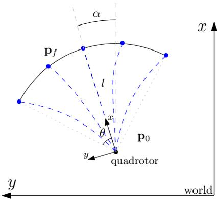
Fig. 5: Trajectory generation. We uniformly sample  $N$  points on an arc, defined by  $\theta$  and  $l$ , in front of the quadrotor. The candidate trajectories are shown in blue.  $\alpha$  is the yaw angle of the quadrotor.
