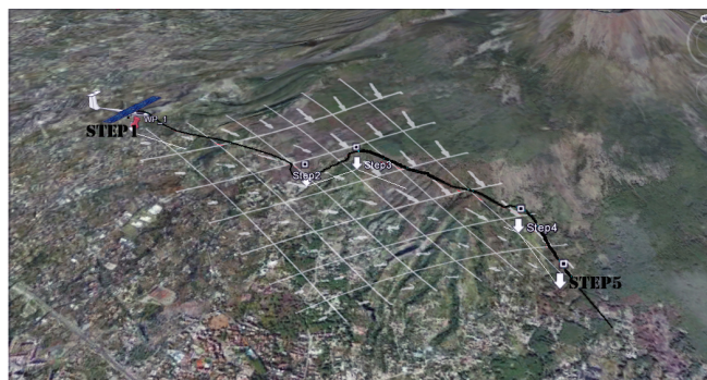
Fig. 1. A planned path that exploits wind energy from the start point (step1) to the target point (step5).
