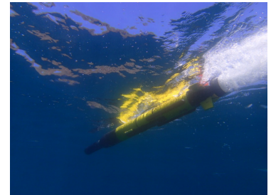
Figure 1: YSI EcoMapper Autonomous Underwater Vehicle executing a mission off the coast of Santa Catalina Island.
