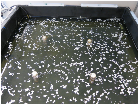
(a) An image of the mCoSTe testing tank at Drexel University with tracer particles floating on the water surface.
