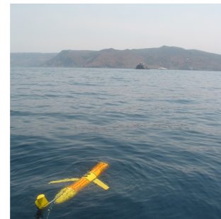
(b) A CINAPS [5] Slocum glider preparing to start a mission off the Northeast coast of Santa Catalina Island, CA.
