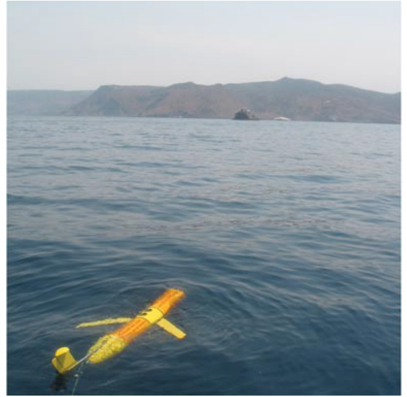
Fig. 8. A Slocum glider preparing to start a mission.
