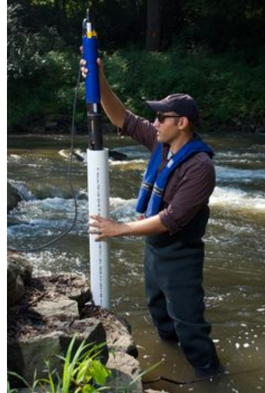
Fig. 3. University of Virginia Multiparameter Eulerian Water Quality Meter is shown [4].
