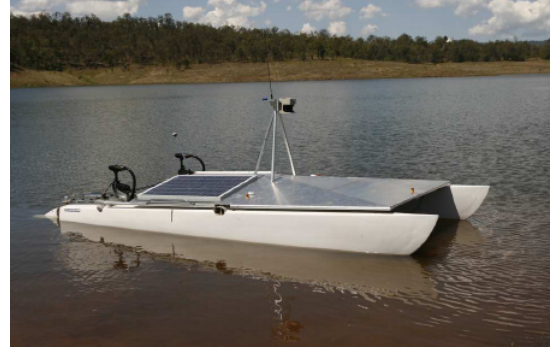
Fig. 5. Solar Powered Autonomous Surface Vehicle [7].
