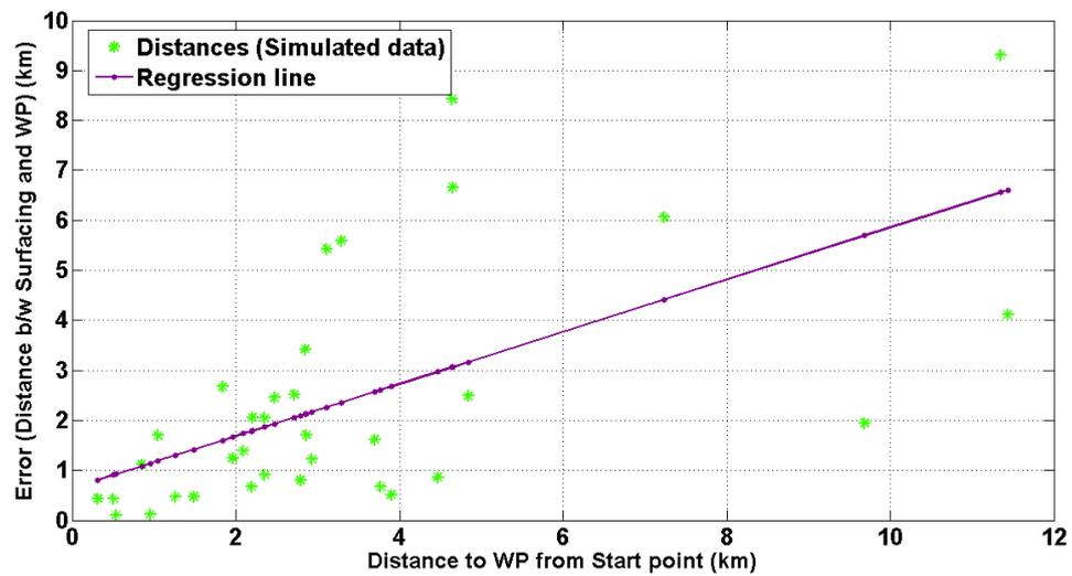
Figure 5. A plot of the absolute surfacing error (in km) versus the length of the prescribed trajectory for the simulated trials.
