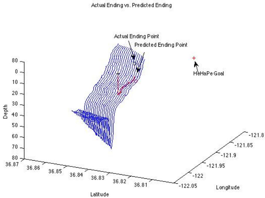
Figure 10. Final results comparing the predicted ending point and the actual ending point. The prescribed goal location is also plotted, demonstrating the more than 4000m dead-reckoning error.
