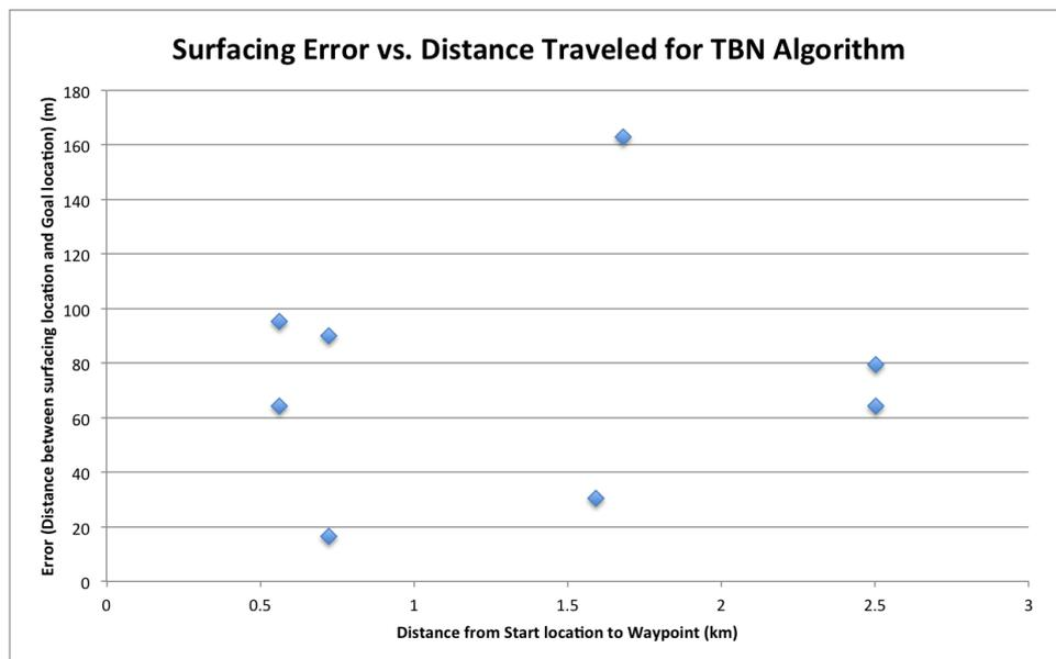
Figure 12. A plot of the TBN predicted surfacing error in meters versus the length of the prescribed trajectory in kilometers.
