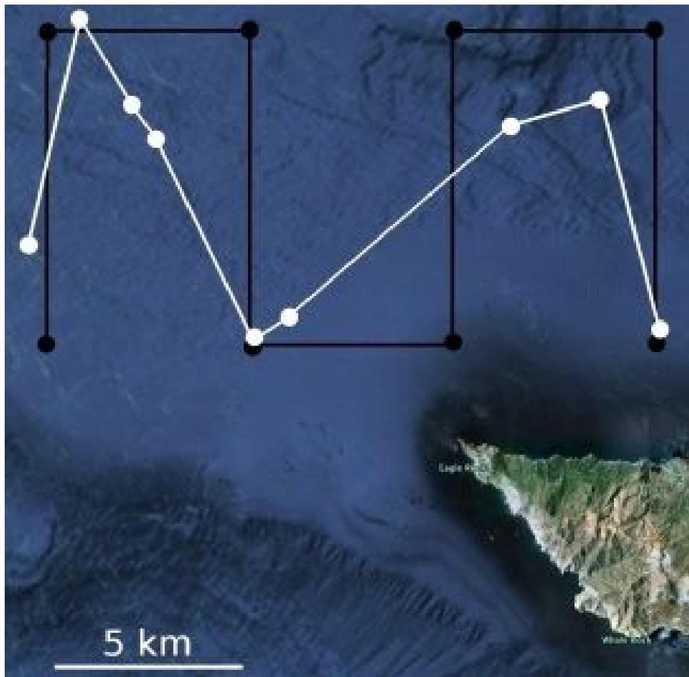
**Figure 1.** Planned lawnmower pattern (black waypoints and path) and the actual executed path (white surfacing locations and path) for a glider deployment off of the northern tip of Santa Catalina Island, CA.
