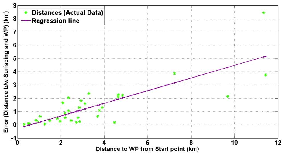
Figure 3. A plot of the absolute surfacing error (in km) versus the length of the prescribed trajectory for the actual field trials.
