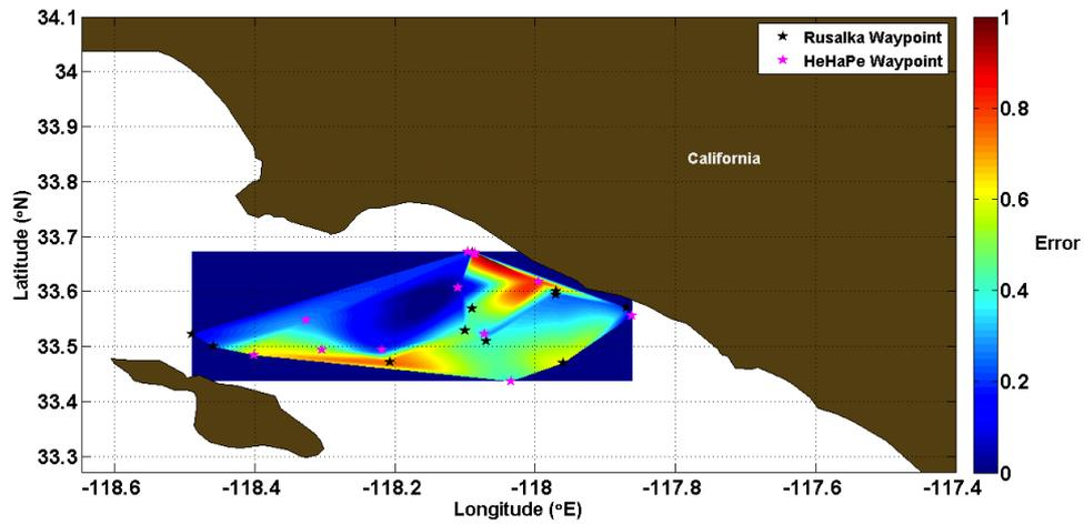
Figure 4. A heat-map surface plot representing the normalised error between the surfacing location and the prescribed waypoint for the actual field trials.
