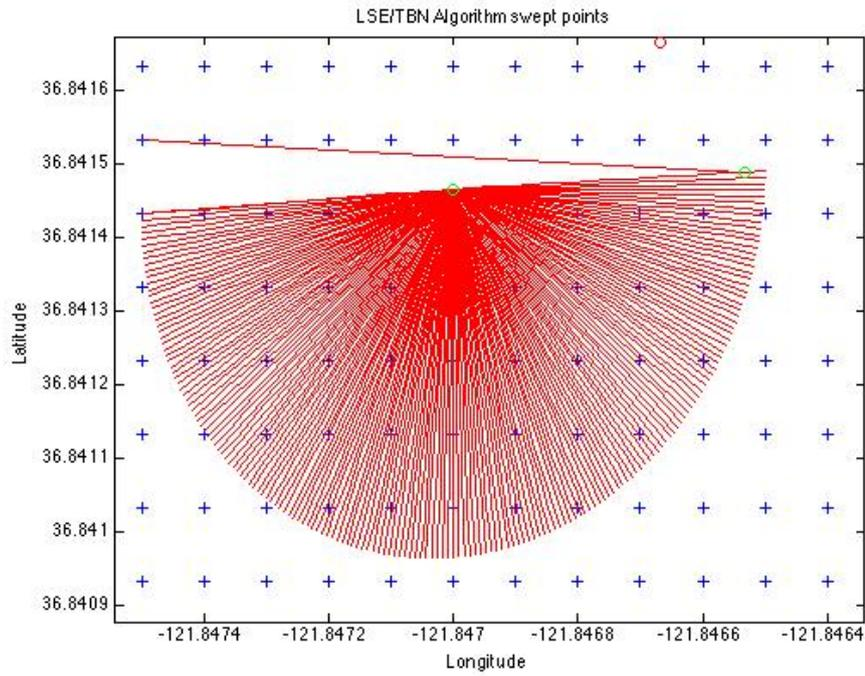
Figure 9. Path options generated around the start Latitude and Longitude. 180 path options are shown in red.
