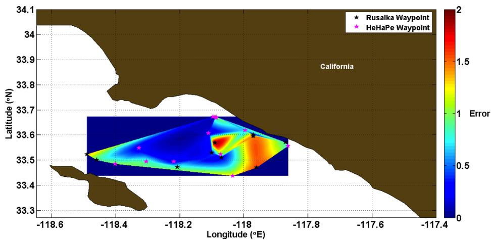
Figure 6. A heat-map surface plot representing the normalised error between the surfacing location and the prescribed waypoint for the simulated trials.
