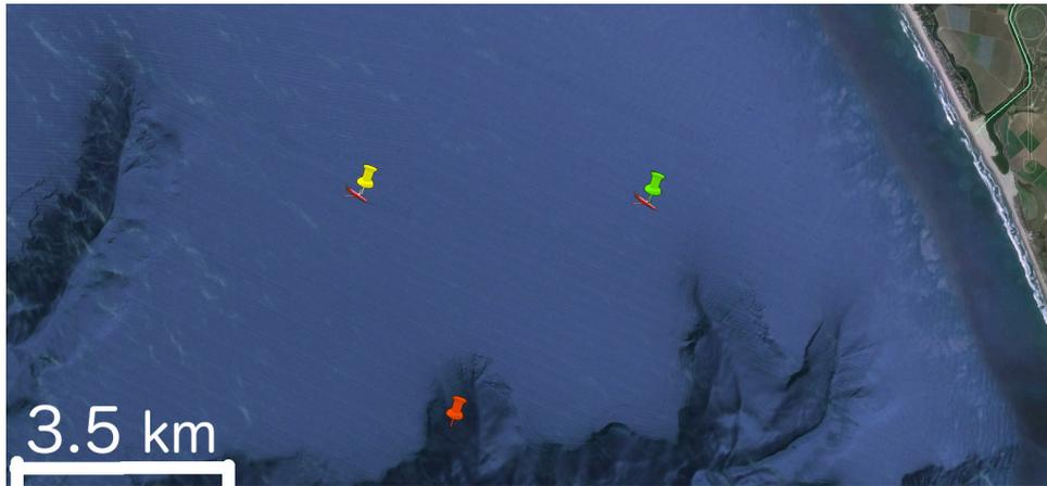
**Figure 7.** The start position and end position are the yellow and green pins on the map, respectively. The goal position of the glider is the red pin on the map. The straight line (inaccurate) path of the glider is assumed to connect the yellow pin and the green pin. Image courtesy of Google Earth.
