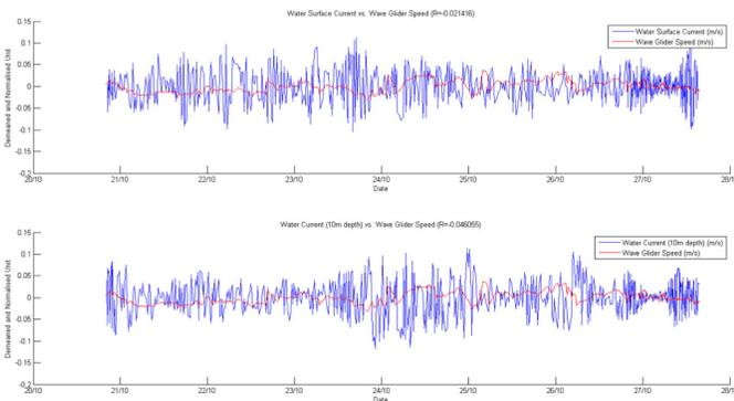
Figure 6: Correlation between Wave Glider Speed and water current speed input parameters during the Monterey Bay field trial.
