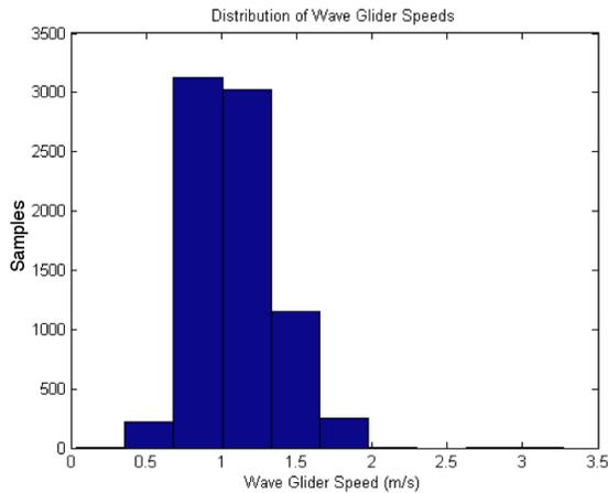
Figure 3: Distribution of Wave Glider speed during the Hawai'i field trial.
