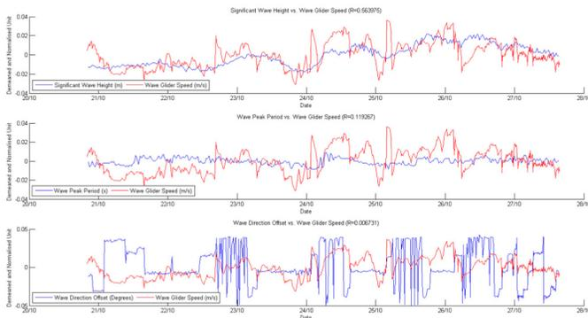
Figure 5: Correlation between Wave Glider Speed and wave input parameters during the Monterey Bay field trial.
