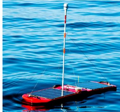
Figure 1: The Wave Glider platform.
