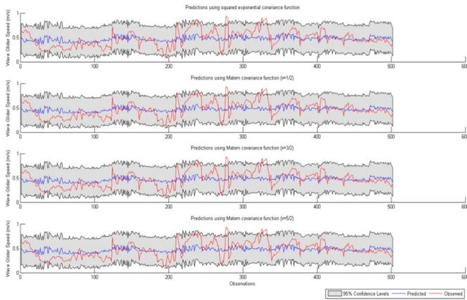
Figure 8: Predicted versus actual Wave Glider speeds from Gaussian process models using different covariance functions during the Monterey Bay field trial.
