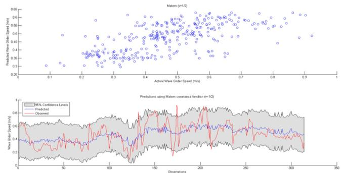
Figure 9: Predicted versus actual Wave Glider speeds from Gaussian process models using different covariance functions during the Monterey Bay field trial.
