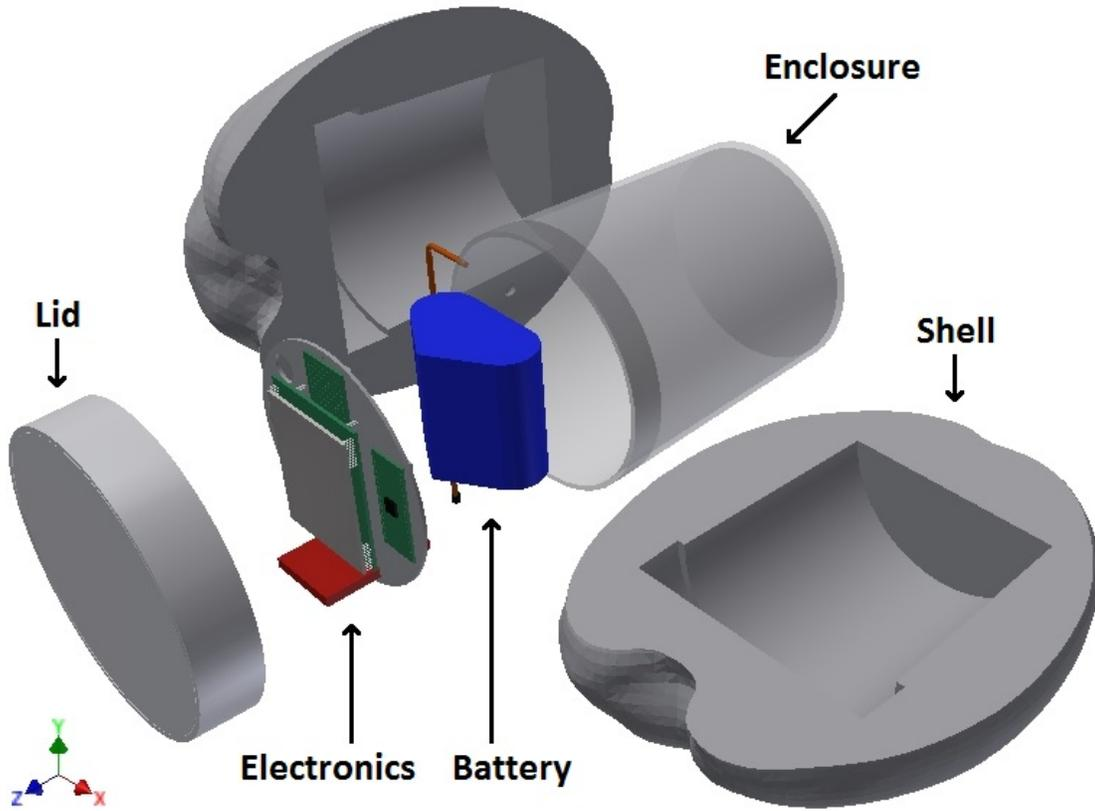
Fig. 4: Exploded view of electronics, battery, polycarbonate housing, and *pseudoseed* shell.
