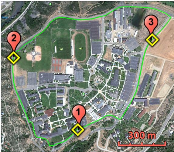
Fig. 8: Location information gathered along a path from the SPOT Connect device overlaid on a Google Maps image. The diamonds represent specific locations of the device, with the red pins the recorded GPS location.
