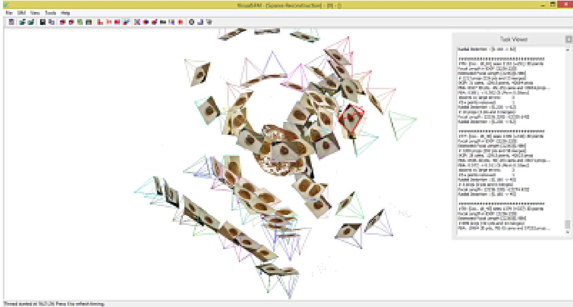
Fig. 6: Visual SFM sparse 3D reconstruction process.
