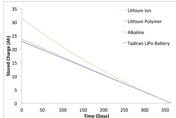
Fig. 11: Discharge profile of various battery designs. Note that the Alkaline battery profile is hidden underneath the Tadiran discharge line.
