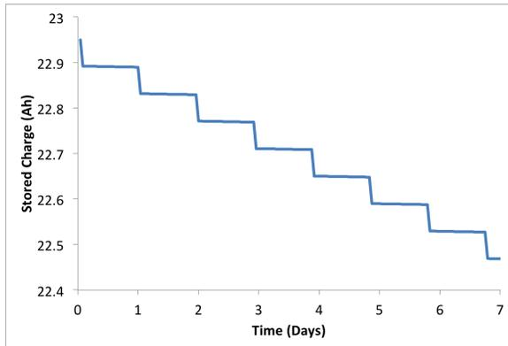
Fig. 10: Estimated power discharge profile of a battery over the period of one week.
