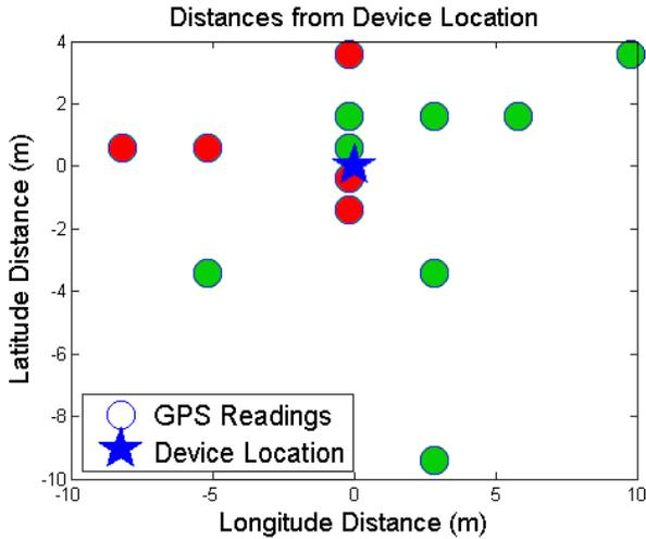
Fig. 7: Distance from the actual location of the device to the recorded GPS reading. The different colors (red and green) represent data collected on separate days.
