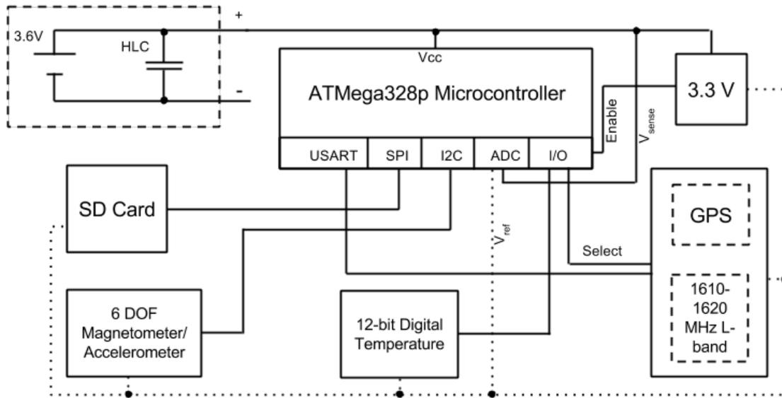
Fig. 9: *Pseudoseed* function block diagram at subsystem level.
