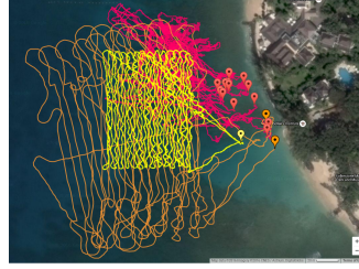
Fig. 3. The GPS traces of the three different kinds of vessels: Drifters red, ASV yellow, AUV orange.
