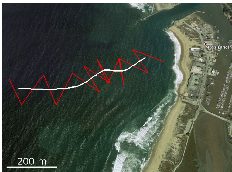
Fig. 5. A delineation of the chosen Monterey Canyon depth contour as the initial prior for the pseudo-front (white). The initially computed path for the AUV is the zig-zag path shown in red.
