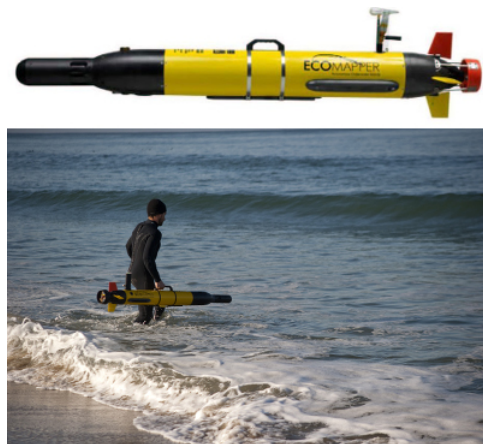
Fig. 3. The YSI Ecomapper Autonomous Underwater Vehicle (top), and the beach deployment of the vehicle (bottom).
