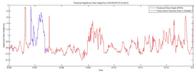
Fig. 10. The WAVEWATCH III predictions of significant wave heights throughout the Wave Glider mission using time and Wave Glider position.
