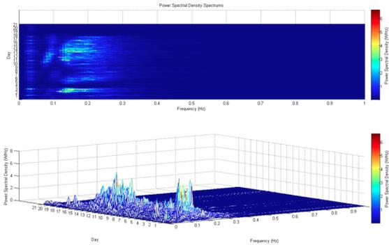
Fig. 4. Power spectrum densities measured by the Wave Glider during the Hawaii field trial.
