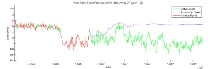
Fig. 13. Forecasted Wave Glider speed k-step iterative Gaussian process method (Lag = 100).
