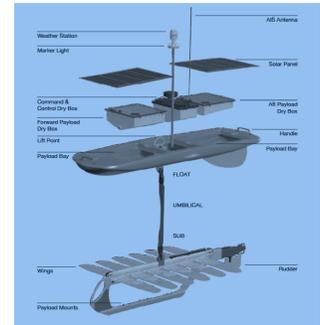
Fig. 2. Architecture of the Wave Glider platform.
