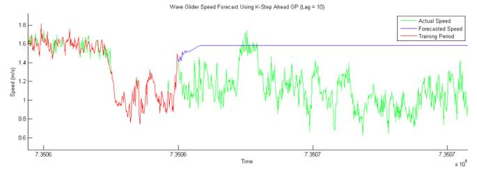
Fig. 12. Forecasted Wave Glider speed k-step iterative Gaussian process method (Lag = 10).
