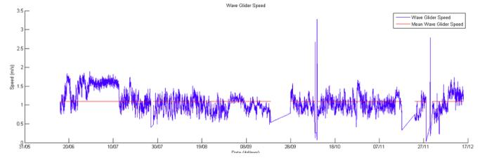
Fig. 9. Wave Glider speed for the entire duration of the six-month Hawaii deployment.
