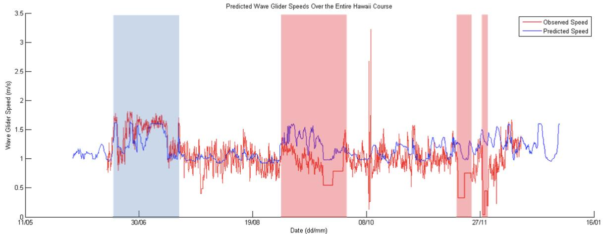
Fig. 15. Wave Glider speed forecasted with WAVEWATCH III data from a model trained on the Datawell wave spectrum data.
