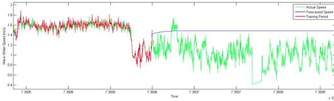
Fig. 11. Forecasted Wave Glider speed using the periodic covariance function.
