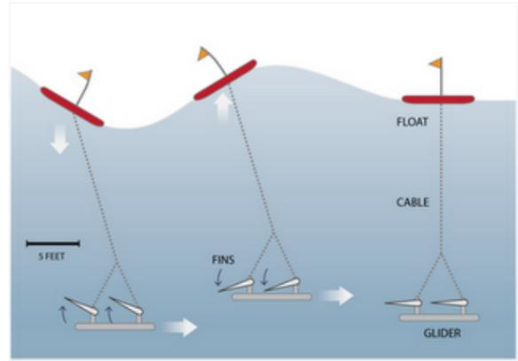
Fig. 3. Basic operation of the Wave Glider platform.
