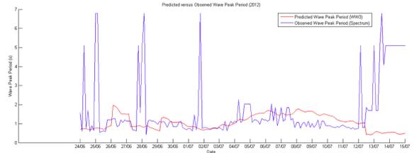
Fig. 6. Predicted and observed wave peak periods from WAVEWATCH III and estimated from spectral data collected on-board the WG, respectively.
