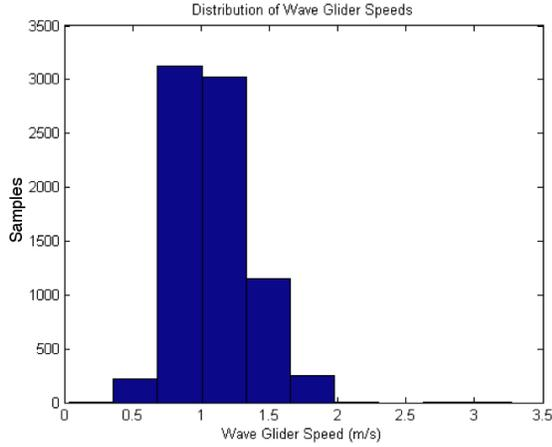
Fig. 7. Distribution of Wave Glider speed during the Hawaii field trial.
