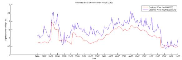
Fig. 5. Predicted and observed significant wave heights from WAVEWATCH III and estimated from spectral data collected on-board the WG, respectively.
