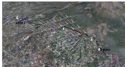
Fig. 1. A planned path that exploits wind energy from the start point (Step1) to the target point (Step5). While Step 2, Step 3 and Step 4 are the locations where the UAS changes the heading angle to follow the prescribed path.
