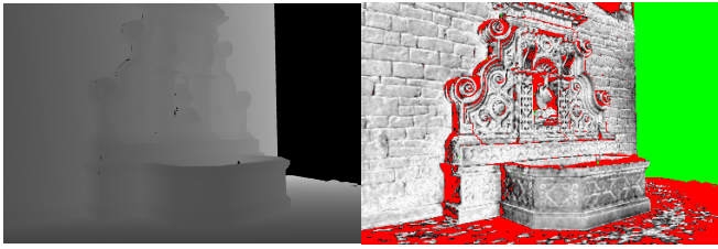
Fig. 3. (left) Example image of the rendered ground-truth depth-map for the fountain sequence. (right) An example of the error statistics gathered during the experiments, green denotes no ground-truth measure, red a gross error ( > 10\sigma ), white no error increasing towards black ( 10\sigma ).
