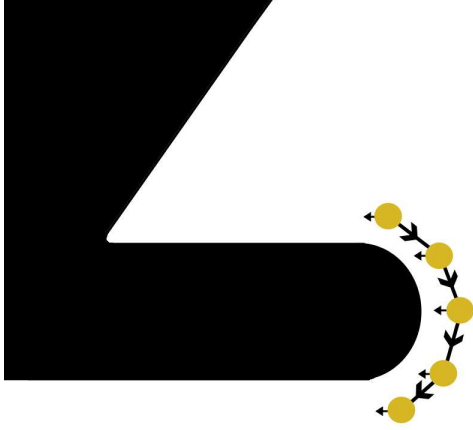
Fig. 5. Side view of a bulbous bow on a ship. Also pictures is the semi-circle trajectory for the inspection of the front of a bulbous bow.
