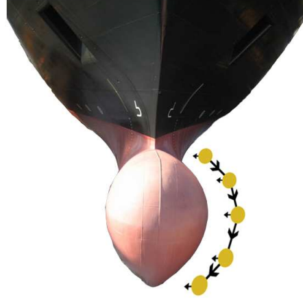
Fig. 6. Front view of the bulbous bow of the M/V Eurodam. Also depicted is the trajectory to survey the sides of the bulb. Picture modified from Rijkaart (2008).
