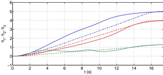
Fig. 3. State trajectories for the position vector:  $\eta_1$  (blue),  $\eta_2$  (red),  $\eta_3$  (green). The solid line represents the trajectory obtained via the PWC control synthesis while the dashed line is the time-optimal trajectory.
