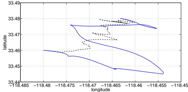
Fig. 6. Reference trajectory projected to the sea surface (dashed black line) and the computed PWC trajectory (solid blue line) trajectory with eight switchings projected to the sea surface.
