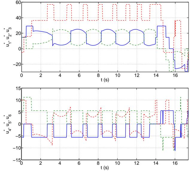
Fig. 1. Time-optimal control signals from [7]:  $u_1^*$  (solid blue),  $u_2^*$  (dashed red),  $u_3^*$  (dot-dashed green) in the top plot;  $u_4^*$  (solid blue),  $u_5^*$  (dashed red),  $u_6^*$  (dot-dashed green) in the bottom plot. In [7, Fig. 2], the corresponding signals for the eight thrusters are shown, where they are computed using a static control allocation.
