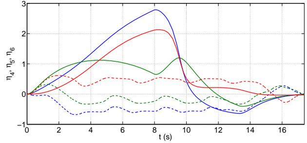
Fig. 4. State trajectories for the orientation vector:  $\eta_4$  (blue),  $\eta_5$  (red),  $\eta_6$  (green). The solid line represents the trajectory obtained via the PWC control synthesis while the dashed line is the time-optimal trajectory.
