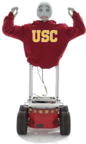
Fig. 1. The Bandit upper-body humanoid robot.
