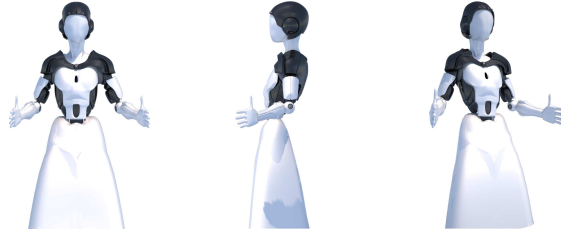
Fig. 1. Quori, a modular social robot platform for human-robot interaction.
