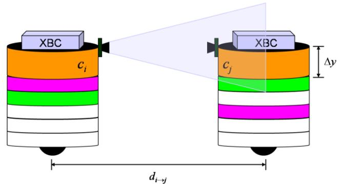
Fig. 10:  $c_i$  identifies the “face” of  $c_j$  and determines its relative distance; note the orange band is always the top band.
