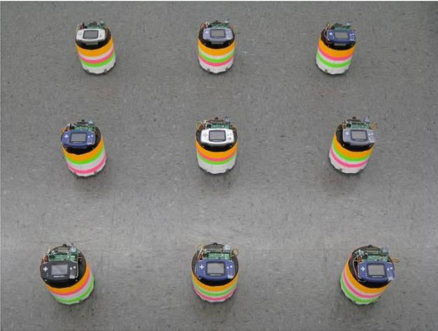
Fig. 11: Top formation:  $f_1(x) = 0; f_2(x) = x \sqrt{3}; f_3(x) = -x \sqrt{3}; R = 24.0$ ". Bottom formation:  $f_1(x) = x; f_2(x) = -x; R = 24.0$ ".
