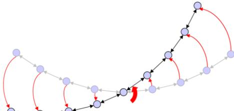
Fig. 4: A formation rotation command sent to a seed cell rotates the entire formation.
