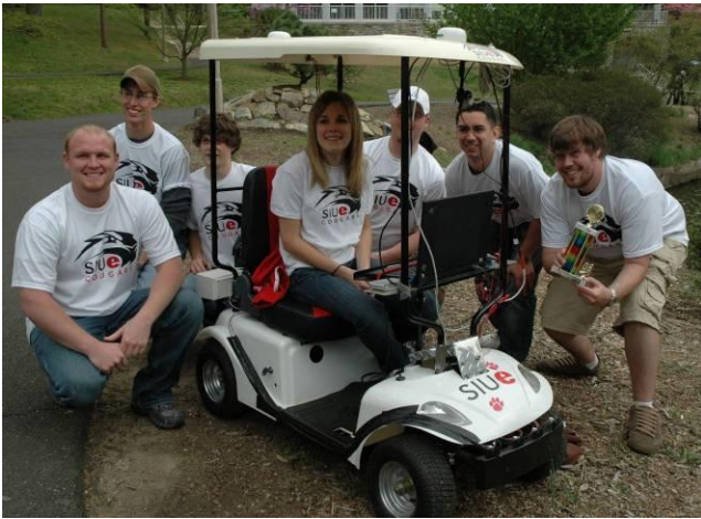
Figure 2: Robotics team with completed retrofitted cart. Note that the driver space is maintained with clear access to the laptop.
