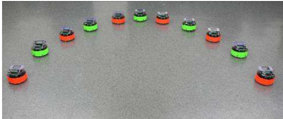
Figure 10: Eleven robots in a parabolic formation defined by the geometric description F \leftarrow f(x) = x^2 .
