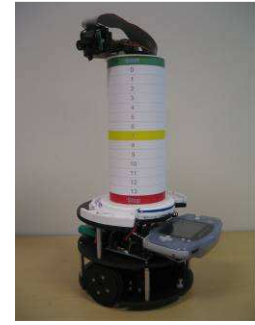
Figure 10: Color bar-coding system (left) implemented on a robot prototype (right).
