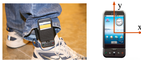
Fig. 3: Position of the phone for data collection with the axis
