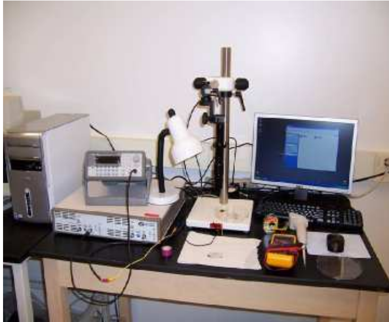
Figure 6.3: Electronic setup for manual activation of electrodes.
